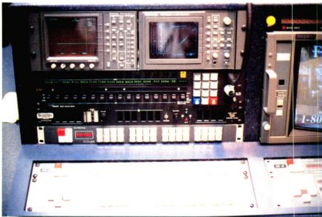
Maintenance of digital systems will be more centralized than ever. Test stations like the one shown here will concentrate sophisticated test equipment at one location where signals can be carefully analyzed.
