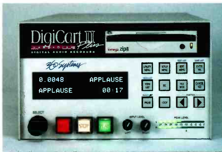
Tape-based cart machines are a thing of the past for any new audio studio. Shown here is the 360 Systems DigiCart II Plus hard-disk recorder, which provides the old-style cart portability with all the advantages of digital storage.
