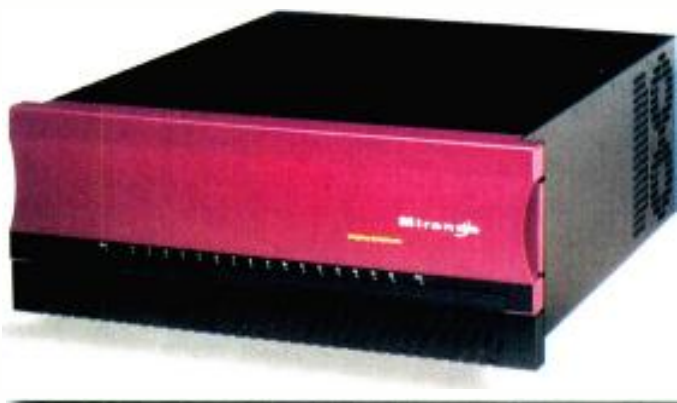
In most new TV audio installations, just monitoring and routing the audio will be a big problem. New solutions based on an integrated housing, coupled with a variety of plug-in cards, are now available from companies like Miranda, which showed the new Symphonie at NAB. The card frame holds 16 audio or video function cards.
