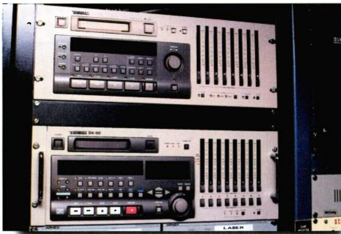
For some applications, only a double system of recording will provide enough audio tracks. Shown here are a Tascam DA98 and DA88 eight-track recorders.
